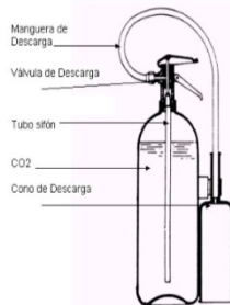
EXTINTOR DE: GAS CARBONICO
